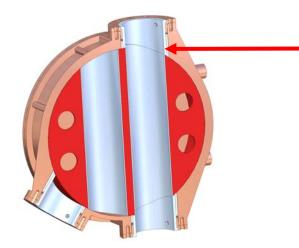
Capsulated high thickness pipe: in stainless or hardened steel for food compatibility or more resistance against wear
